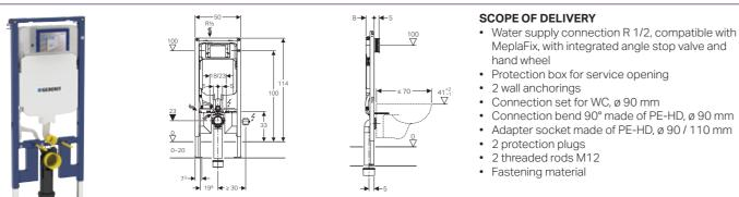
Duofix mounting element for wall-hung WC front operated for actuator plates "Sigma80, Sigma70, Sigma60, Sigma50, Sigma30, Sigma20, Sigma01".
