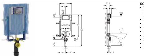
SCOPE OF DELIVERY • Water supply connection R 1/2, compatible with MeplaFix, with integrated angle stop valve and hand wheel Protection box for service opening • 4 fixing brackets • Connection set for WC, ø 90 mm
